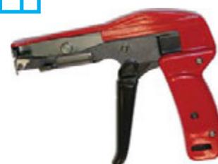
**TRONCHESI PER FASCETTE DI CABLAGGIO IN NYLON** (cable ties cutters)
