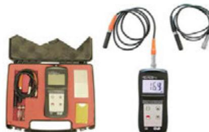
**MISURATORI DI SPESSORI A ULTRASUONI** (ultrasonic thickness meters)
