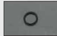
Inverter Spot HSS Steel 2+2 mm
