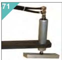
71 XS3200 VELOX 350 Morsa pneumatica ver- ticale. Vertical pneumatic vice.
