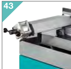
BS 300/60 - BS 300 PLUS Morsa pneumatica. Pneumatic Vice.
